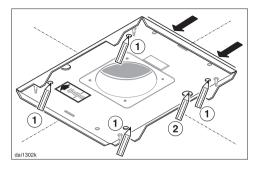
■ Hold the mounting plate up to the ceiling so that the orange arrow faces the front of the hood and aligns with the lines drawn on the ceiling. Mark the position of the four mounting bolts ① for securing the mounting plate and determining the position of the hole the power cable ② will pass through.
